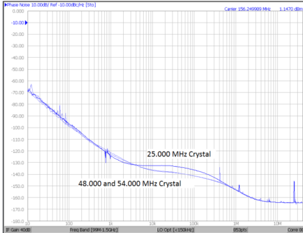
Figure 2. Si5345 156.250 MHz Phase Noise Comparison Using 25.000, 48.000, and 54.000 MHz Crystals as the XA/XB Reference
