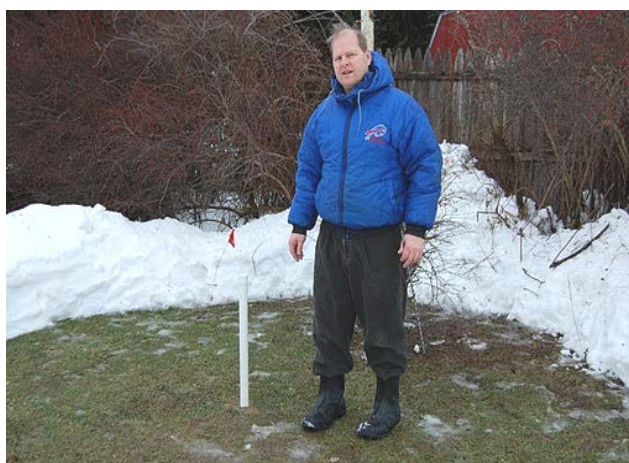
Figure 3. A frost tube (outer PVC casing showing) in a snow cleared area at Site 2.
