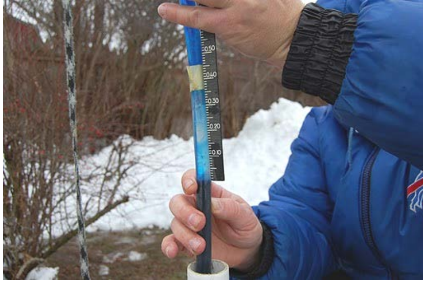
Figure 1. Frost tube measurement showing a frost depth of 8.8 cm (3.5 in.). The lower edge of the tape indicates ground level.
