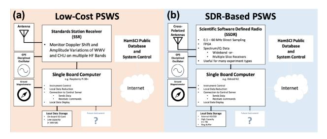
The research needs can be met with the development of two variants of the PSWS: a low-cost entry-level model, and a higher-cost model with more capabilities. It should be noted that TAPR development currently is focusing on the (b) higher performance SDR-based PSWS.
